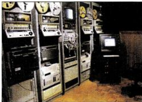
Cyphertech is using its encoding equipment to place digital data in the audio portion of TV programming.
